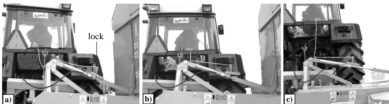
Fig. 17. Mechanical lock of hydraulic lifting function
